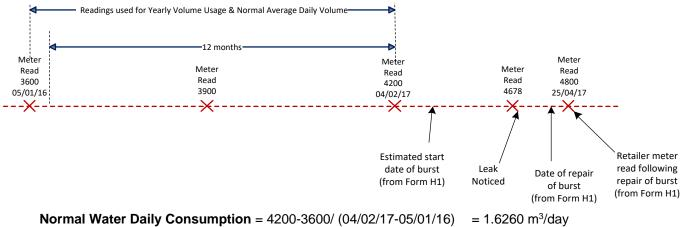
**Leakage Duration** = 25/04/17 - 04/02/17= 80 days  $= 600 \text{ m}^3$ **Total Water Consumption** = 4800 - 4200
