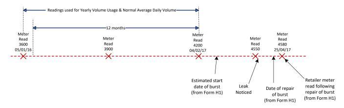
Normal Water Daily Consumption = 4200-3600/ (04/02/17-05/01/16)  $= 1.6260 \text{ m}^3/\text{day}$ **Leakage Duration** = 25/04/17 - 04/02/17= 80 days **Total Water Consumption** = 4580 - 4200 $= 380 \text{ m}^3$ Normal Water Consumption = 1.626 x 80  $= 130 \text{ m}^3$  $= 260 \text{ m}^3$ **Double Normal Water Consumption** Leakage Volume = 380 - 130  $= 250 \text{ m}^3$
